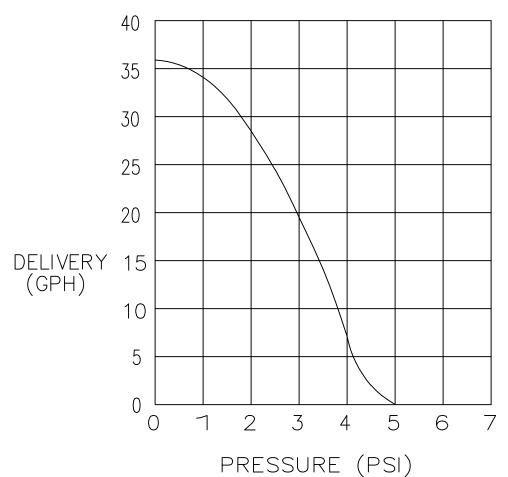
DELIVERY VS PRESSURE. TYPICAL CURVE AT RATED VOLTAGE. ZERO
